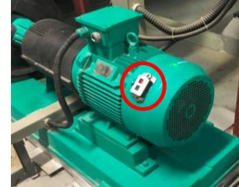
Use sensor instead of manual to collect equipment condition indicator, to reduce or eliminate machine down risk.
